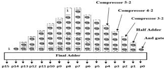
Fig.13.Signed Wallace tree multiplier using Proposed Compressors
